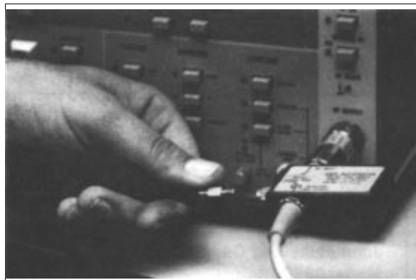
Figure 1-8. Example Use of Compensation Washer with WSMA Connectors
